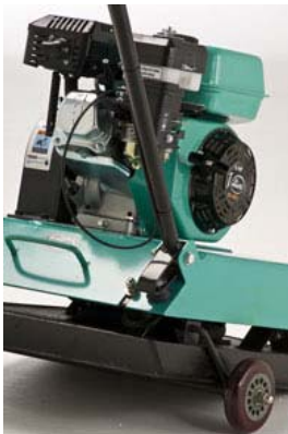
showing oil bath air cleaner and extra muffler bracket
